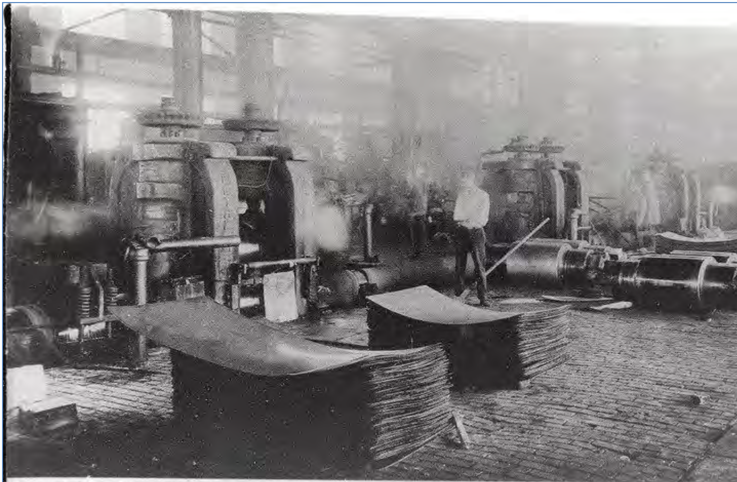
An additional set of 12 hot mills was added in 1920, and a third set of 12, shown here, came on in 1925, making a total of 36. Two years later, in 1927, the addition of 12 more mills brought the total to 48 and the capacity to 4,250,000 base boxes, or 210,000 tons, annually. Two employees (blurred on mill at left) worked each mill — a feeder and a catcher. These mills are marked "Bethlehem."
