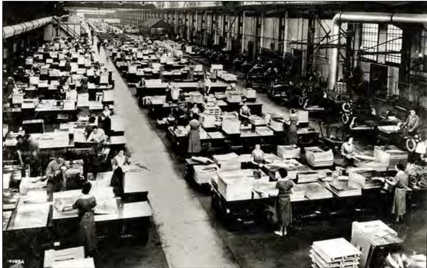
The Tin Room where the “tin floppers,” 200 per shift, worked, checking each sheet of tin plate for defects by “flopping” it over during World War II.
